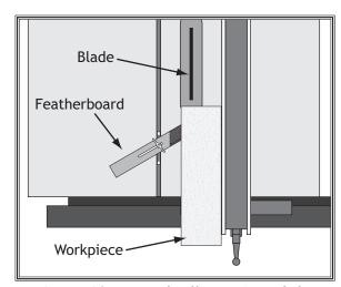
**Figure 68.** Example illustration of the featherboard mounted in the miter slot.
